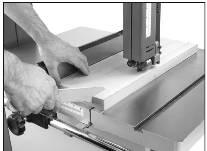
Figure 39. Ripping with a push stick.
